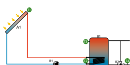
Internal heat exchanger, intelligent pump control, heating return increase
