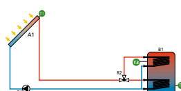
Internal heat exchanger, zone loading, intelligent valve control, intelligent pump control
